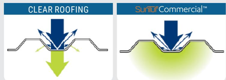
Suntuf Commercial provides a 180 degree spread of light that is brighter compared to clear and tints. The bright light provides unique energy saving properties, making it ideal for farm sheds/workshops without a power source.
